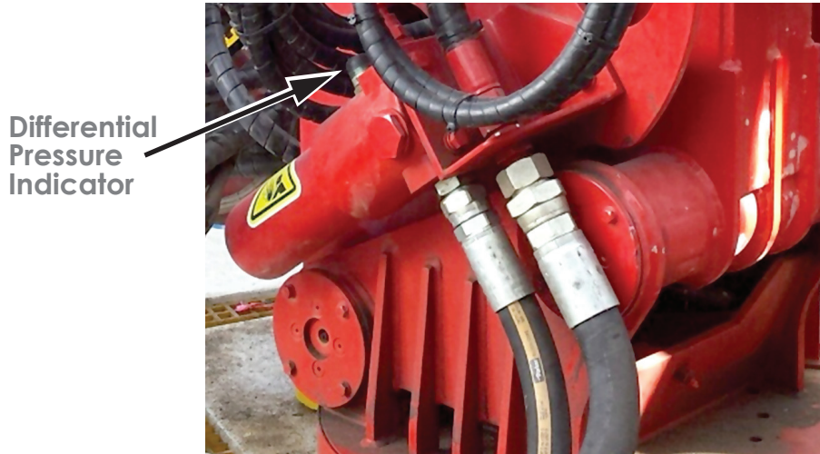
Figure 4: The Differential Pressure Indicator Turns Red to Indicate the Need for Changing the High-Pressure Oil Filter
