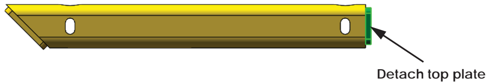
Figure 8: Grind the weld to detach top plate
